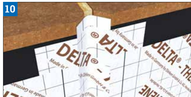
Joint de dilatation (Fig. 10)
